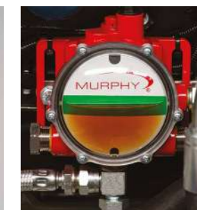
Oil level monitoring system
